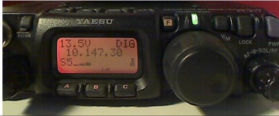
The Yaesu FT-817 is an allmode portable transceiver. It provides 5 watts output which i.e. on 30 m is absolutely enough to be heard. (fits cigarette lighter socket) Unlike FSK frequency setting is less sensible; so go straight to 10.147,30 kHz.
