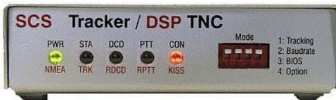
The tracker is simply connected by a **6-pin mini-DIN** (both sides !) male plug to the YAESU. For configuration USB connection is provided for a notebook. If using UI-View KISS red LED eluminates.
